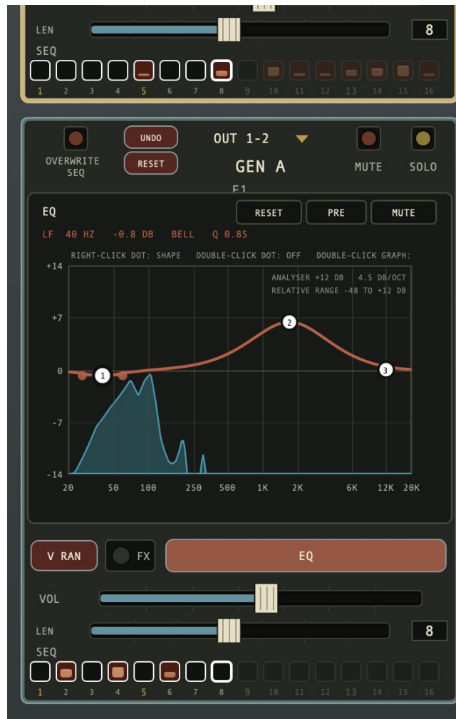
GEN A three-band curve and continuously updating spectrum analyser.
